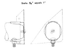
646514 Track End Cap with bolt and nut. Galvanized. Two needed per track run. Packed 20 per carton with mounting bolts. Wt. of Pkg. 6 lbs. 646515 End Trim. Bird proofs the space between the track and cover and serves to finish off the cover ends. Two recommended for each run of track. White enamel. Packed 20 per carton with mounting screws. Weight of package 6 lbs.
