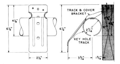
Track and Cover Bracket. For mounting a single run of Track and Cover on a track plank. One required for each 2-feet of track run. Shape of bracket and cover allows plenty of room for both vertical and lateral door adjustment. Galvanized. Packed 50 per carton. (One package handles 100-feet of track). Weight of package 20 lbs.
