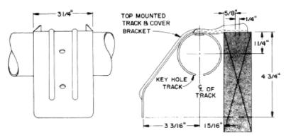
Top Mounted Bracket used with a single run of Track and Cover. Top Mounted on a 2-inch track plank only. One bracket required for each 2 feet of track run. Galvanized. Packed 50 pieces per carton (one package handles 100-feet of track). Weight of package 25 lbs.
