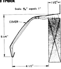
646226 Top Mounted Track Cover. (above) Shaped to fit nominal 2-inch track plank only. Bottom lip hooks over bottom edge of 646519. Track and Cover. Top Mounting Bracket. Top edge flashes junction of track plank and siding. Standard length 10-foot 2-inch. White enamel. Packed 20 pieces per carton. Weight 8 lbs. per carton.
